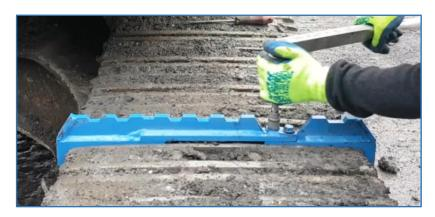
\* TORQUE: M12 SCREWS: 130 NM - M16 SCREWS: 330 NM DAILY CHECK OF GOOD FITTING BEFORE STARTING TO OPERATE
